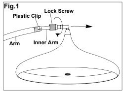
3. Unscrew the lock screw from the arm to slide the inner arm from the arm. (Fig.1)
