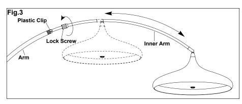
Insert the inner arm into the arm and slide the plastic clip back into the arm to prevent the inner arm from scuffing. Place the inner arm to the desired location and tighten lock screw back to arm. (Fig.3)
