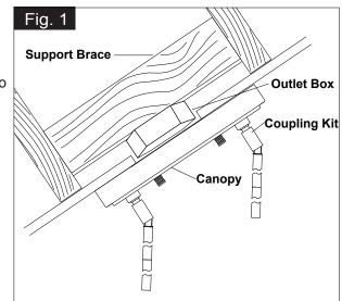
10. Angled mounting recommended for a vaulted or angled ceiling. (See Fig. 1)
